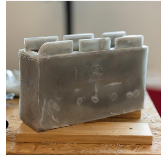
Construction bricks made from recycled plastic takeout containers and beer can carriers at the Innovation Barn [Photo Credit: Charlotte Magazine, August 28, 2022]
